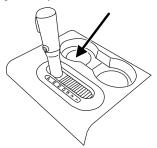
4. Apply the brake and shift into N (Neutral).
